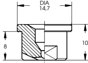
Lubrication of steel strip after cold rolling must be performed by the spray of very low quantities of lubricant, with an outstanding uniform spray distribution. Pnr low-flow flat jet tips, manufactured by high precision machine tools, assure very small tolerance on nozzle capacity and perfect spray pattern.
