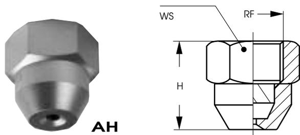
AH nozzles produce a full cone spray pattern, with a very uniform liquid distribution over the entire coverage area. The special design of the internal vane, which do not show any small dimension passage, assures for an excellent resistance to clogging. Based on the above two features, AH series nozzles are widely used in continuous casting plants all over the world and have supplied years of trouble-free service.
