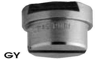
Proper roll cooling assures uniform strip thickness, and requires even water coverage. The even spray distribution of the GY series tips avoids sudden temperature changes and consequent expansion or contraction, which results in the need for roll re-grinding. The final result of a proper roll cooling is then a more even roll wear, longer life, longer production runs with more consistent steel quality.
