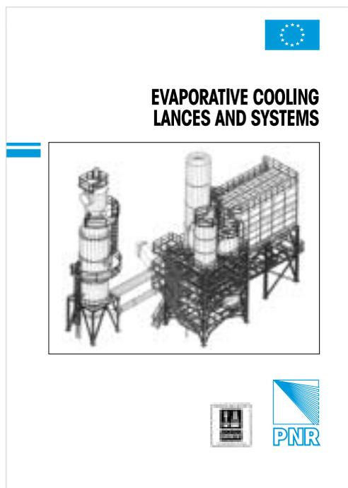
Gas cooling lances serve the purpose of cooling furnace gases prior to their inlet inside the ESP (Electrostatic Precipitator). Our Catalogue **CTG LN14 BR** gives complete information about the gas cooling process and the several types of gas cooling lances. Our offices will be glad to supply any further information and to assist you in the choice of the proper product.
